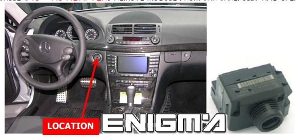
Now remove back plastic cover from EZS, and locate points on the board checking photos belows and solder cable leads as it shows to us: Version 1:
